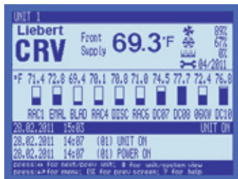
Bar graphs show the inlet temperature of every rack with a 2T temperature sensor.
